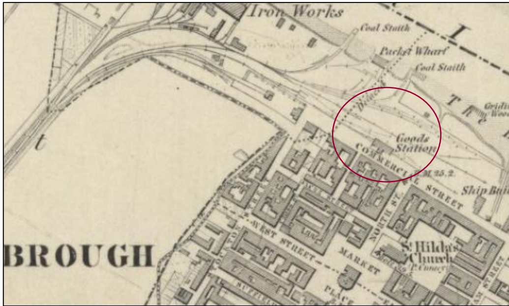
Figure 25. The extended trackbed of 1837 to Commercial Street where a temporary station was provided from 1838 and replaced with a permanent structure in 1839. This was replaced by another station in 1846 and instead converted into a Goods Shed.
